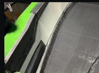
DRY CARBON LAY-UP
