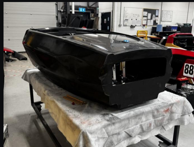
CARBON MONOCOQUE — BUILT IN-HOUSE
