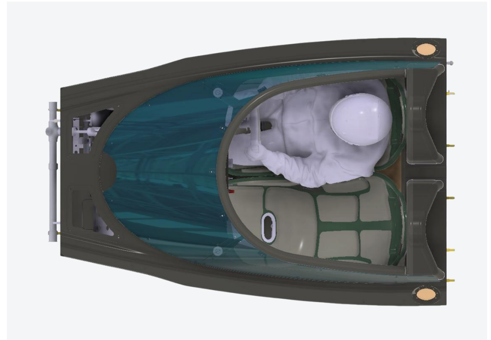
COCKPIT PACKAGING STUDY — TWO OCCUPANTS, PLAN VIEW
